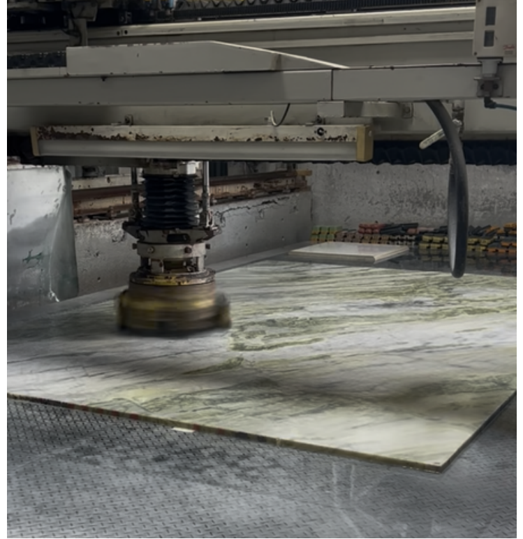
RESURFACER HONING A SLAB OF MARBLE
